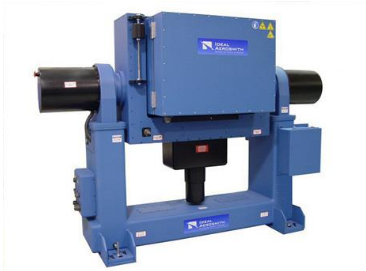
Figure 1: Two-Axis Motion Simulation Table System by Ideal Aerosmith
