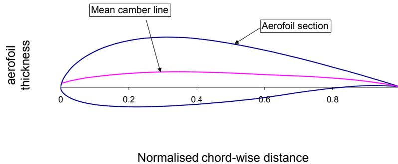
**Figure 3 Mean camber line of an aerofoil**
