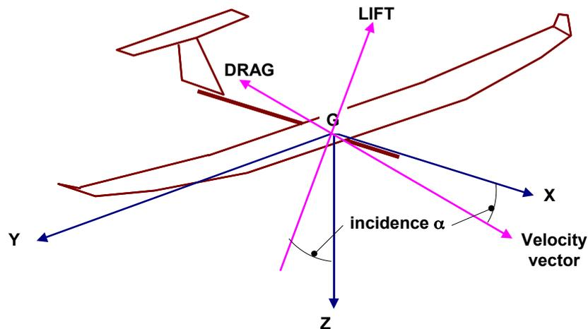
**Figure 4** Wind axes defined
